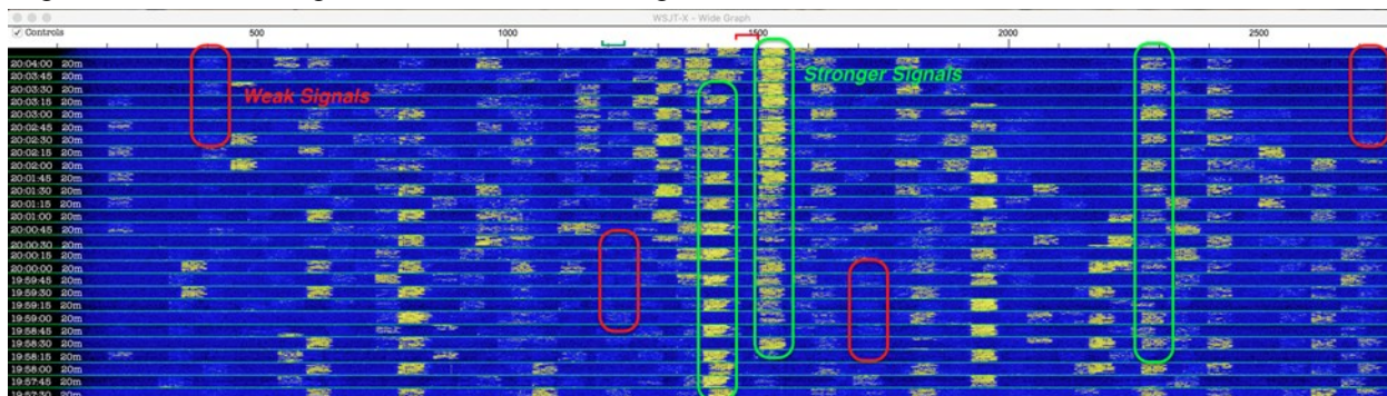
Figure 1 - Weak FT8 Signals Circled in Red, Stronger Ones in Green
