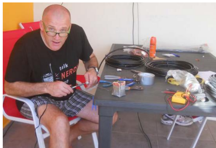
Robert, S53R, making up the phasing lines for the PJ4Q 40m 2-element vertical array.
