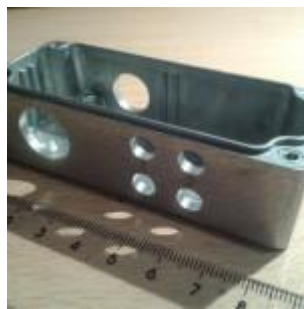
Drilling holes in the case for the connectors and switches.
