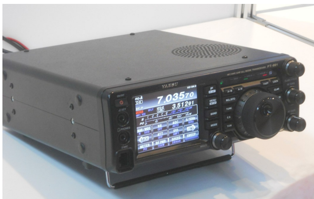
On the Yaesu stand was their new all band (from 160m to 70cm), all-mode transceiver, the FT-991.
