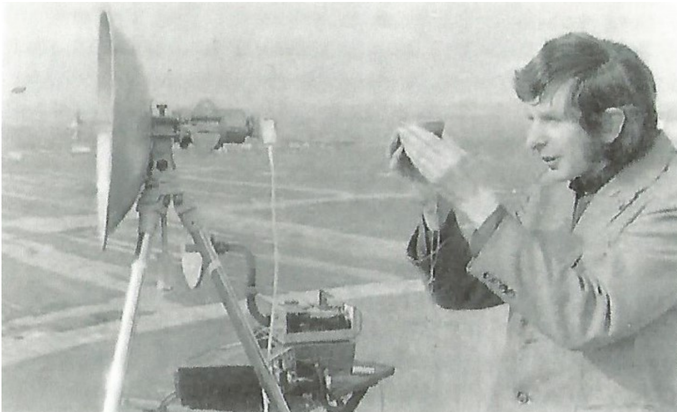
Picture 9, 10 GHz pioneer in Petten using the 3cm wavelength and making a contact with the English station G4ALN on the island Grain. The distance was 310 km!
