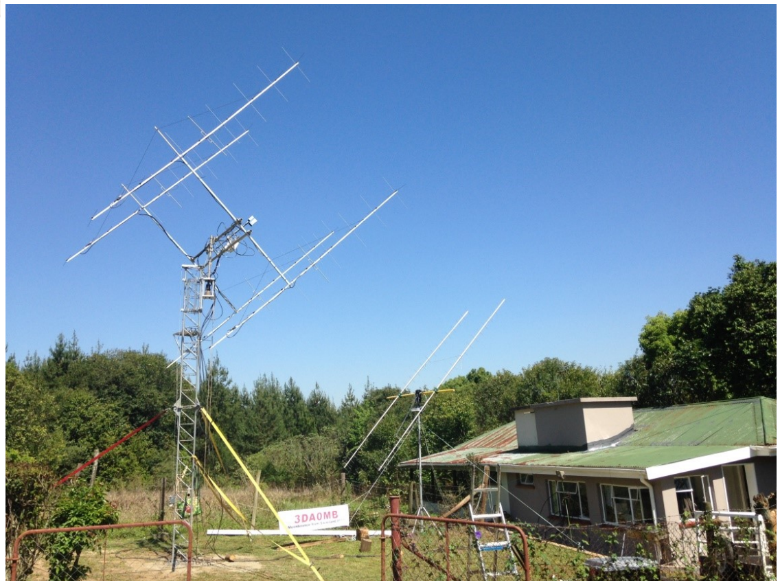
Left 2m array 4 x 9 el horizontal and 4 x 6el vertical design I3DLI, right 70cm 2 x 9WL m2 Hor. or Vert.
