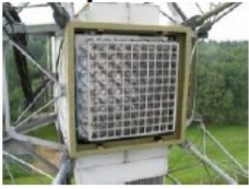
X - polarization: 60 elements Y - polarization: 61 elements
