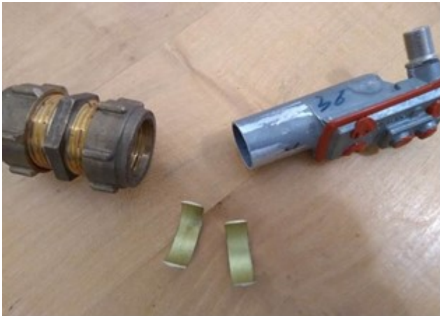
Figure 5 – Compression fitting for a decapitated LNB
