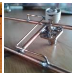
The HB9CV is finished. The small tuning capacitor allows you to get a correct 50 ohm match.
