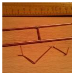
The antenna itself is very small, so the construction needs to be very precise. Using copper wire makes it easy, you can simply solder all parts together, and with a metal file you can get the right measurements.
