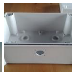
This is the box. I made a hole which will hold the N-connector.
