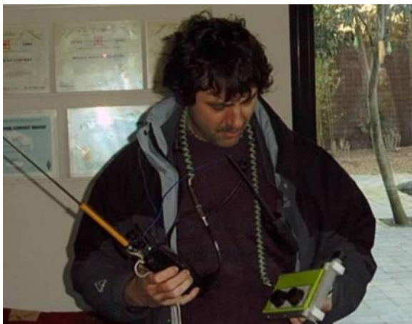
A picture of some of the equipment used to locate RFI-sources. Left hand, an ARDF tracking device for 160m band. Right hand, the SONY ICF-PRO80 receiver.
