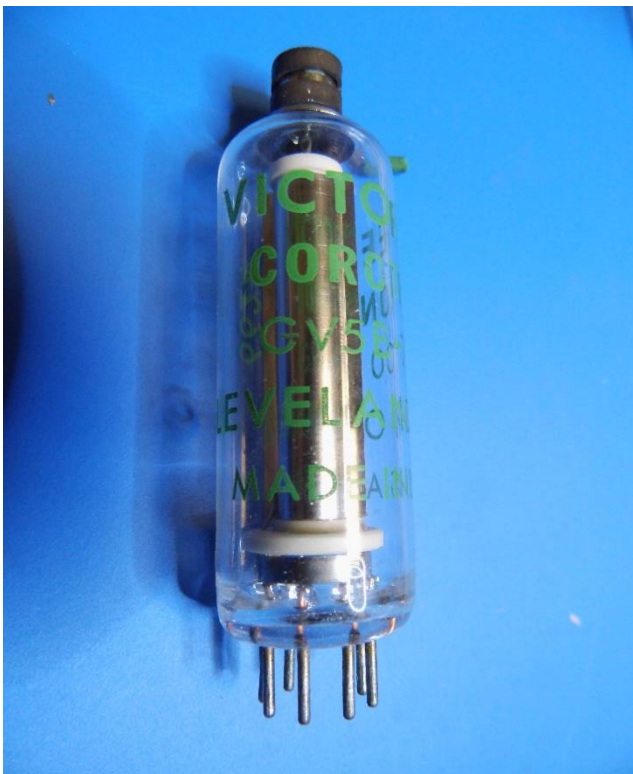
Foto 2, GV5B-700 Victoreen Corotron, corona discharge High Voltage Shunt Regulator Tube 700V nominal at 10 to 450 microamps
