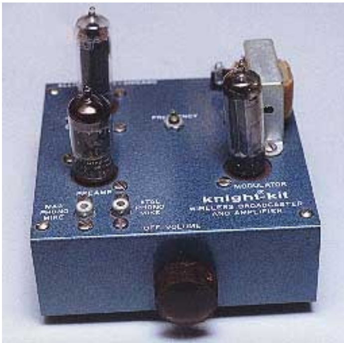
De Allied Knight Kit Wireless AM Broadcaster Low Power AM zender
