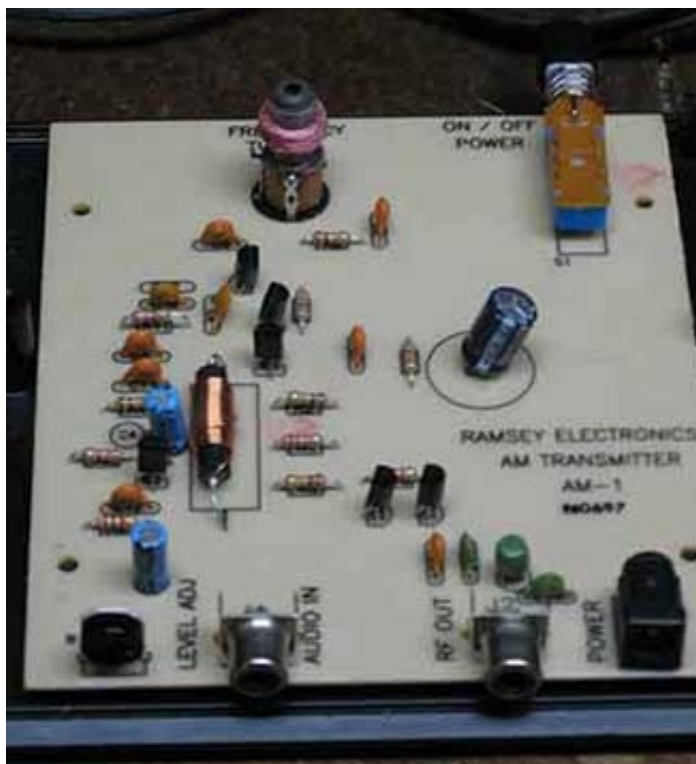
Ramsey Electronics AM-1 AM zender bouwpakket
