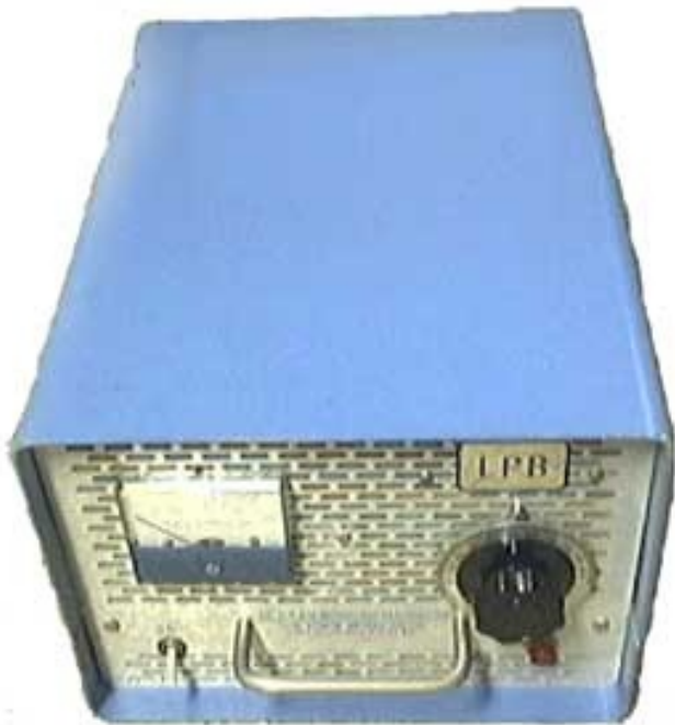
LPB Model RC-25B Carrier Current AM buizenzender
