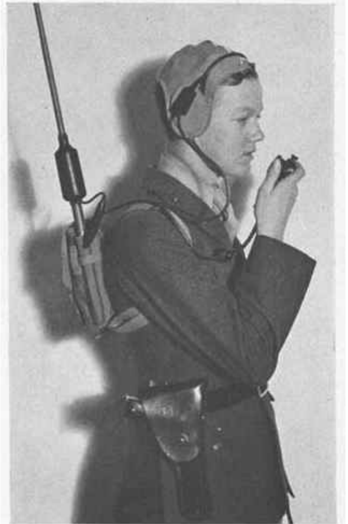
Model MP, MAB transmitting equipment, assembled for operation.
