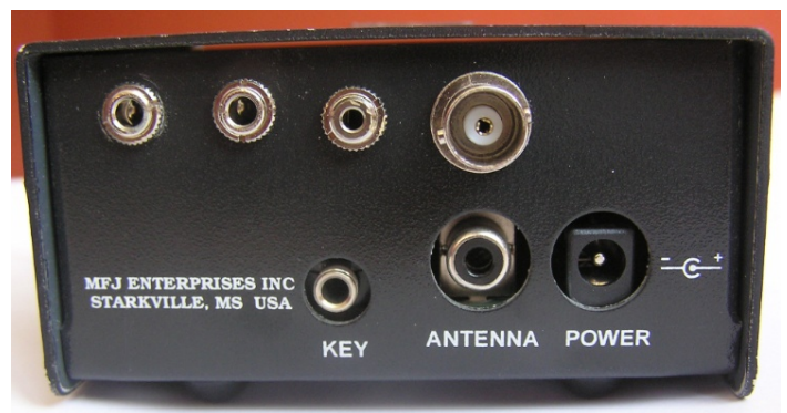
Rear panel with extra in/outputs. The Keyer Output is internally connected to the CUB's key input. So a straight key may still be connected to the CUB.
