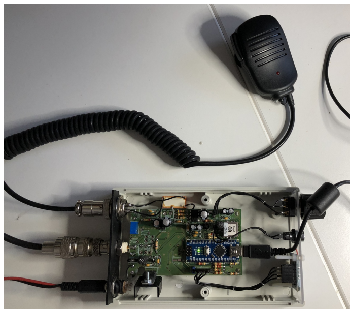
Tracker with 1 channel Voice facility
