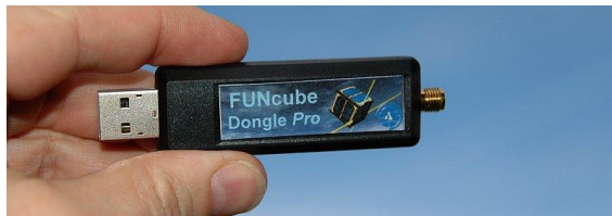
FUNcube Dongle Pro+ is from 150kHz to 1.9GHz
